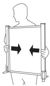
**Note:** Do not touch the screen surface. Handle the MicroScreen only by the case sides or handle.
